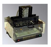
**Type 82C V2.0 Manual Desk Fixture** – This manual desk fixture with **sloping** working area is designed for an ATS-KMFT 670/ATS-MFT 770 with expansion rack. On the rear there are up to **two** (optional) REINHARDT-SR18VG-interfaces.
