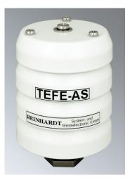
All sensors are designed for outdoor use. They are spray water and rain water tight and are mainly made of high quality steel. The M18-thread on the lower part is for fixing the sensor. It is also the outlet for the cable connection with 3 wires to a 7-pol. socket (ground, supply voltage from 8...20 VDC and output signal from 0 and 5 V).
