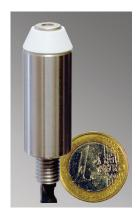
values. Length 50 mm, diameter 15 mm; M8-thread, cable connection with 5 wires (ground, voltage supply, 3 output signals from 0 and 5 V).
